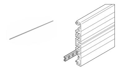
Adapter / Mounting opportunity for fixing of any compents with M3 screws. The threaded insert is slid into the groove of the inside of the side panel.
